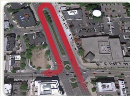
MUT Left Turn Maneuver from a Major Road, Birmingham, MI Source: MUT Video FHWA-SA-14-018
